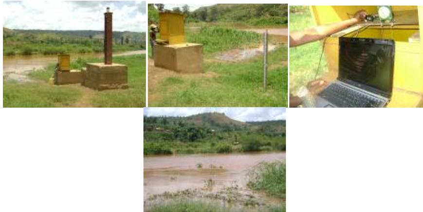
**Figure 5: Gauging station installed at Rusumo for water level measurement of Kagera River.**
