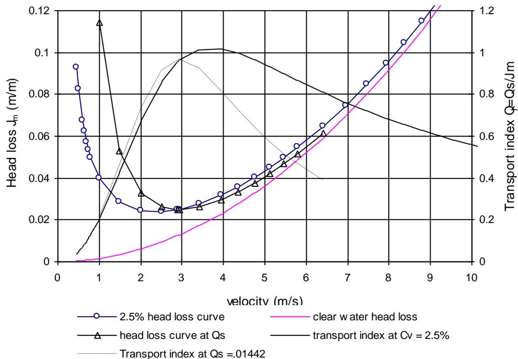
**Fig (5): Head loss and transport index curves at constant  $C_v$  and  $Q_j$**
