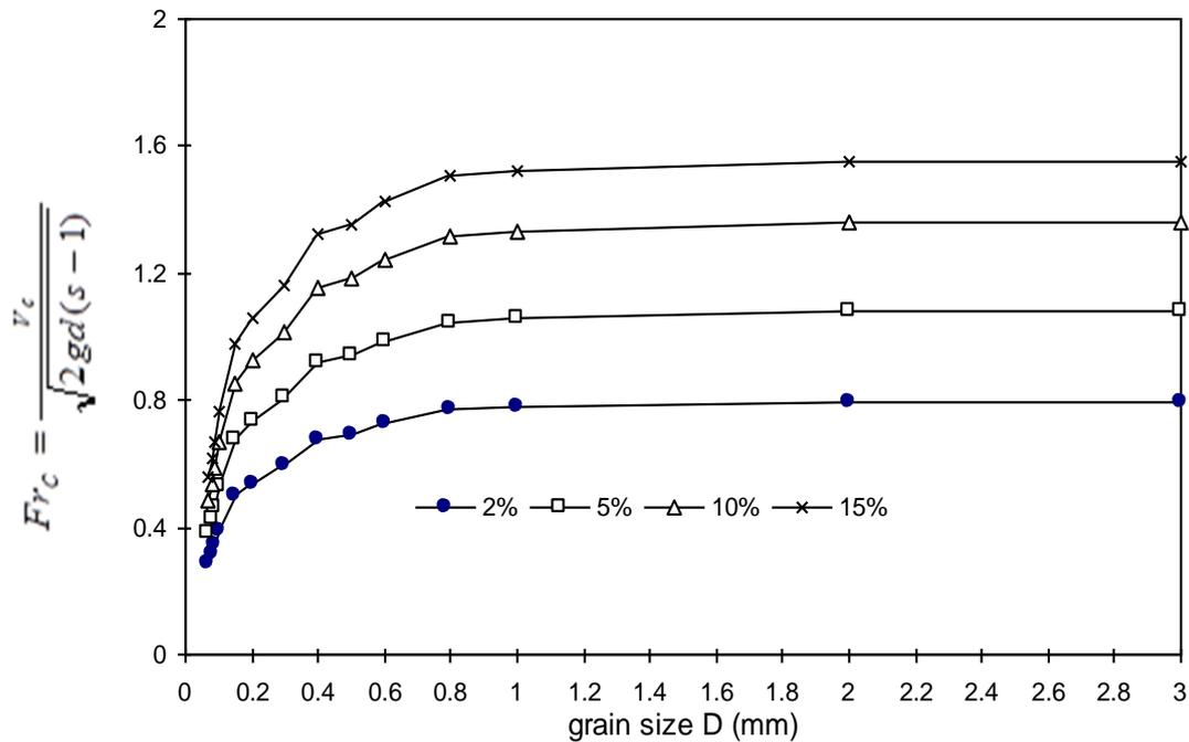
Fig (2): Computed Critical Durand Number Versus Sediment Grain Diameter with Concentration as Parameter
