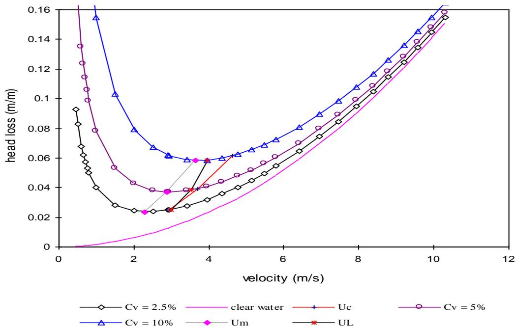
**Fig (4): Head Loss Curves and Critical Velocities  $V_m$ ,  $V_L$ , and  $V_c$**
