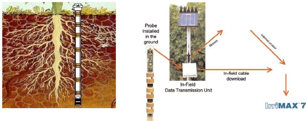
**Figure 5: Enviroscan installation and operation (source: Irrimax7 manual)**
