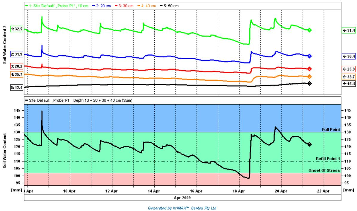
Figure 6: Enviroscan output graph from sensor installed in GR tomato field
