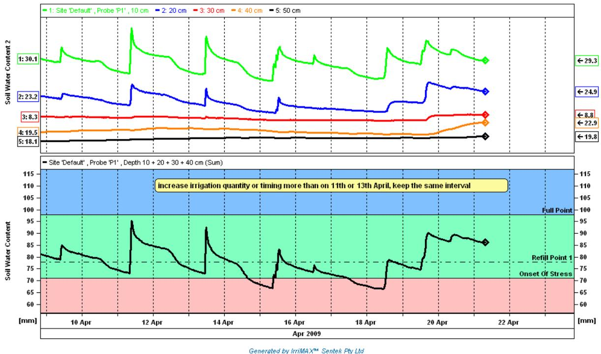
Figure 7: Enviroscan output graph from sensor installed in Eolose tomato field
