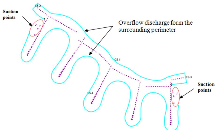
**Figure 4: The locations of the overflow discharge**
