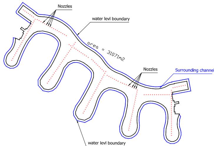
**Figure 3: Lake boundary condition in the design**
