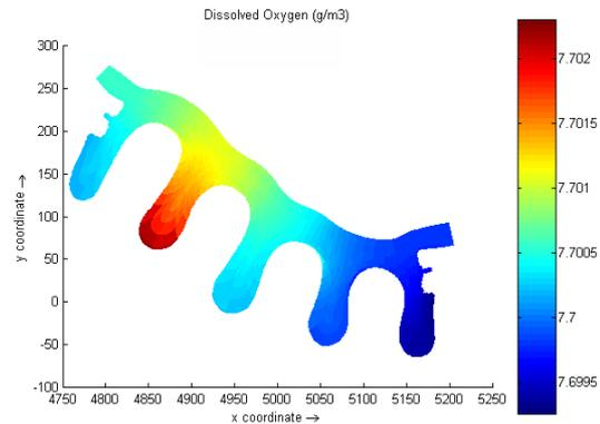
**Figure 8: DO concentration after 48 hrs simulation**
