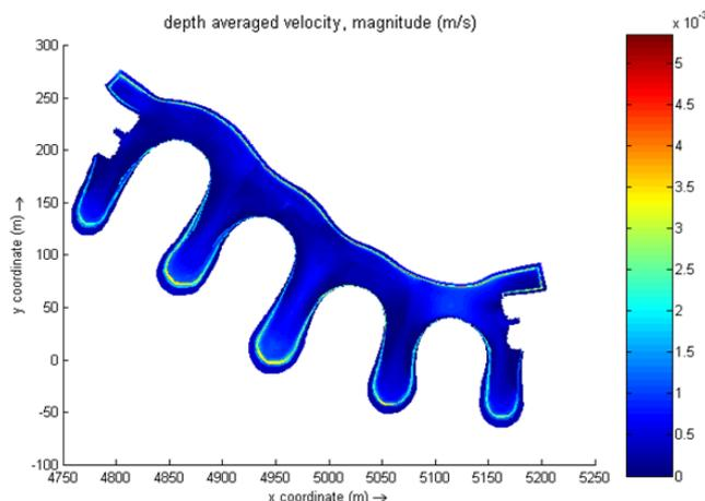
**Figure 5: The depth average flow velocity inside the lake, scenario-3**
