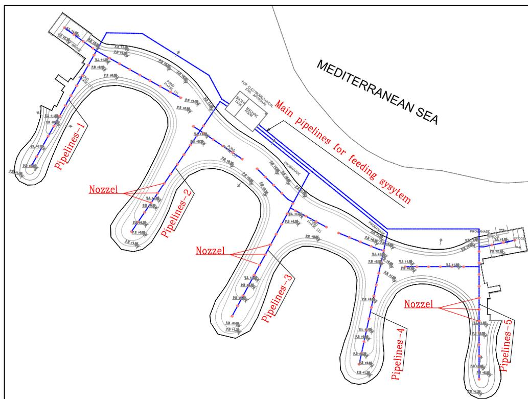
Figure 1: General Layout for the lake and its feeding system
