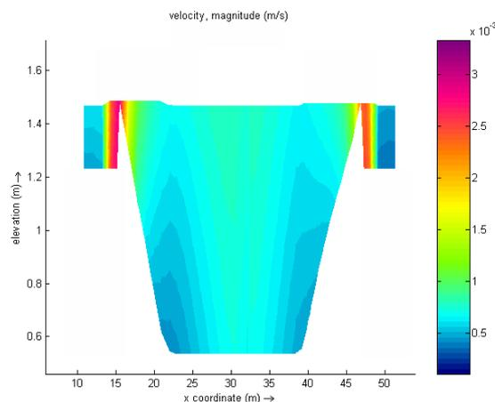
**Figure 6b: Sample of flow magnitude in cross section profile at one finger**
