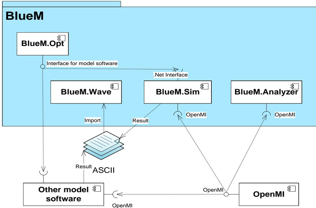
Figure 1: Interfaces of the BlueM Components and Outer Interfaces
