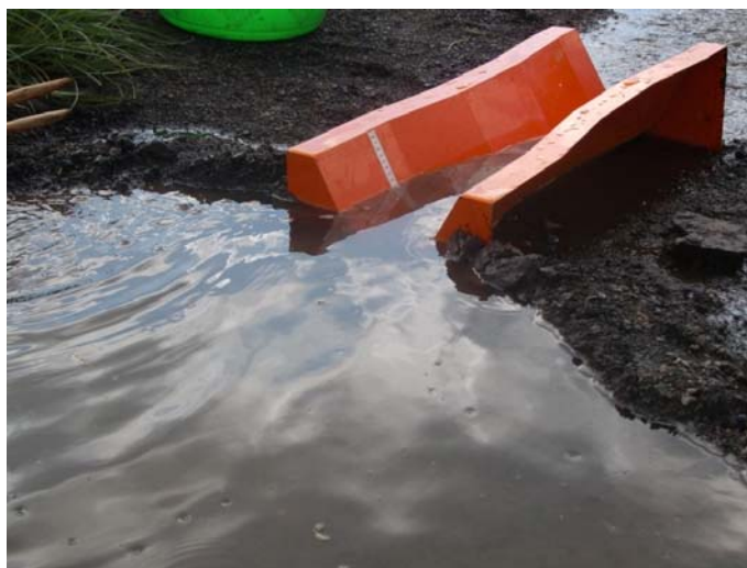
Figure 5: Measurement of stream flow using parshall flume
