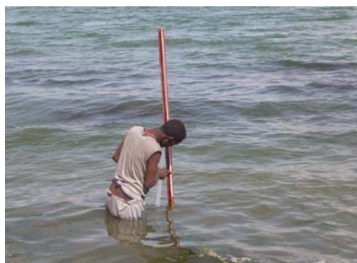
Figure 4: Graduated steel bar installed to monitor the change in water level of the lake
