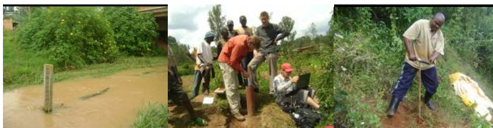
Photo 3: Staff gauge (left), automatic gauging station (center) and piezometer with diver (right).
