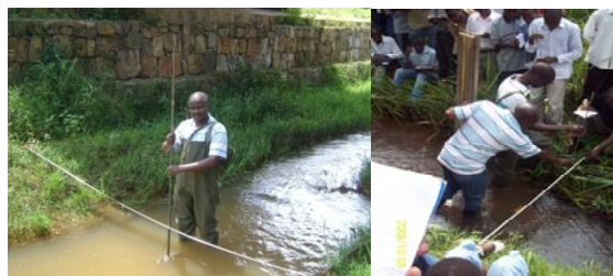
Photo 1: Mukura River discharge measurement (picture taken by Harmen van den Berg on 06/05/2009) and Akagera River discharge measurement (Picture taken on 10/08/2009 by Emille (BSc student) when NUR Civil Engineering students were instructed how to measure discharge using a propeller).
