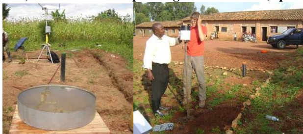
Photo 2: Climate station, evaporation pan, manual and automatic rainfall gauge (tipping bucket) installed in Migina catchment.
