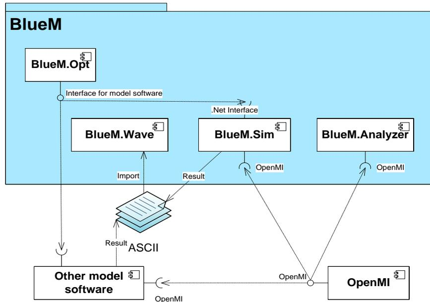
Figure 4: Interfaces of the BlueM components and outer word interfaces
