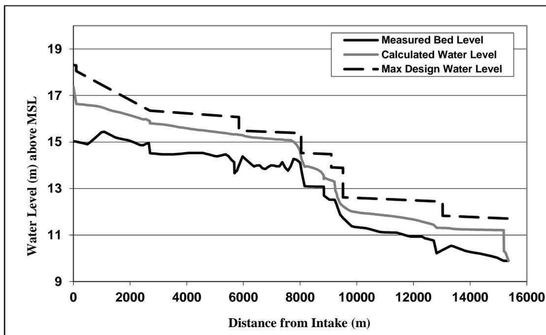
Figure 12: Computed water levels in scenario 4 versus design water levels of Bahr El-Gargaba
