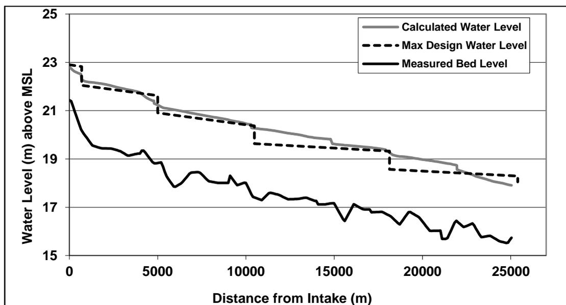
Figure 5: Computed water levels in scenario 2 versus design water levels of Bahr El-Gharq
