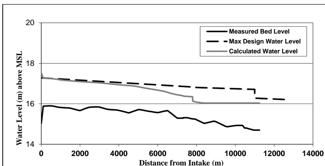
Figure 10: Computed water levels in scenario 3 versus design water levels of Bahr El-Bashawat
