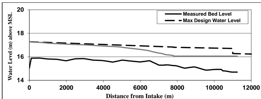
Figure 16: Computed water levels in scenario 5 versus design water levels of Bahr El-Bashawat
