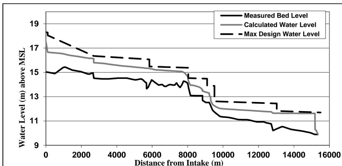
Figure 9: Computed water levels in scenario 3 versus design water levels of Bahr El-Gargaba
