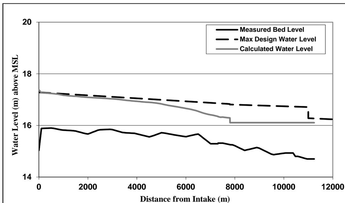
Figure 13: Computed water levels in scenario 4 versus design water levels of Bahr El-Bashawat
