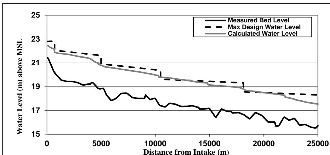
Figure 8: Computed water levels in scenario 3 versus design water levels of Bahr El-Gharq
