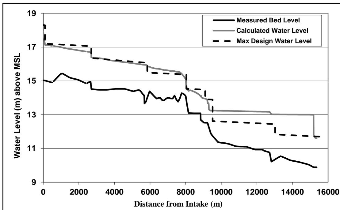
Figure 6: Computed water levels in scenario 2 versus design water levels of Bahr El-Gargaba
