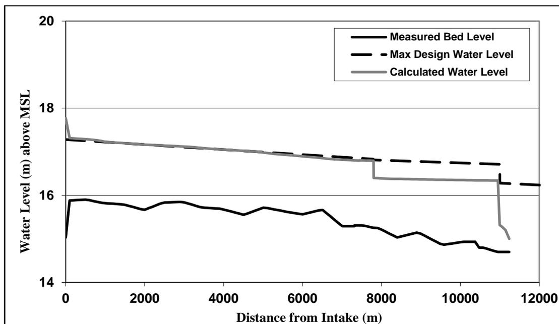
Figure 4: Computed water levels in scenario 1 versus design water levels of Bahr El-Bashawat
