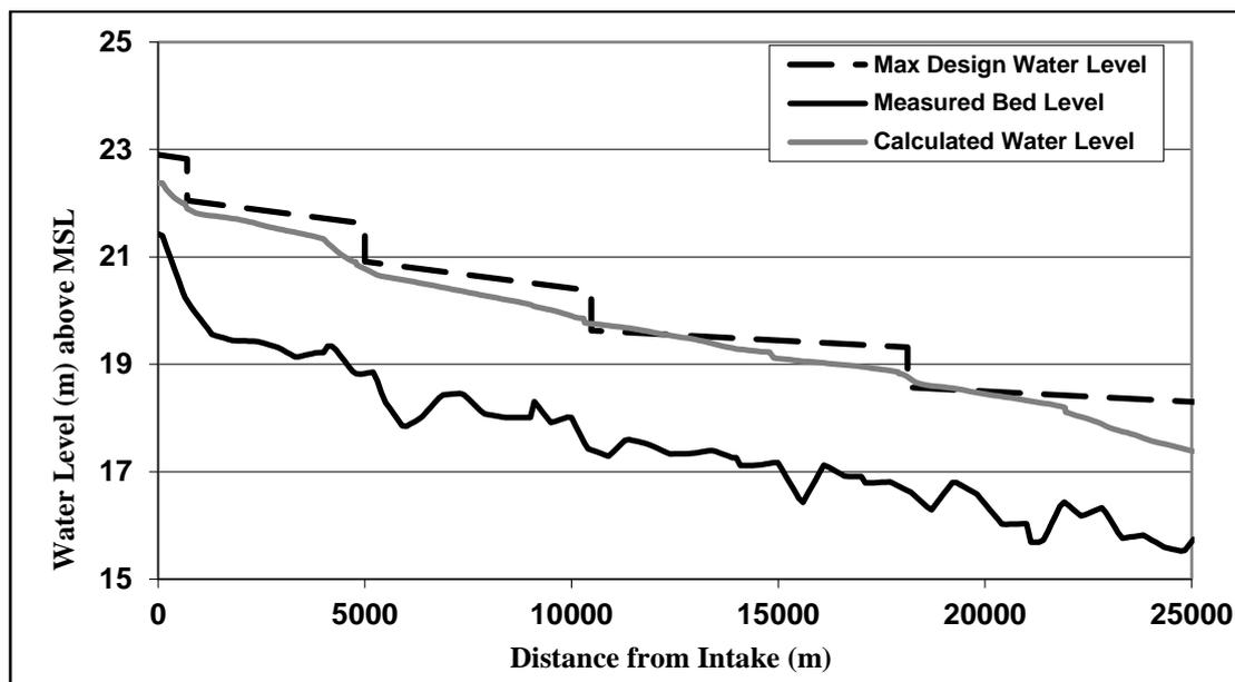
Figure 11: Computed water levels in scenario 4 versus design water levels of Bahr El-Gharq
