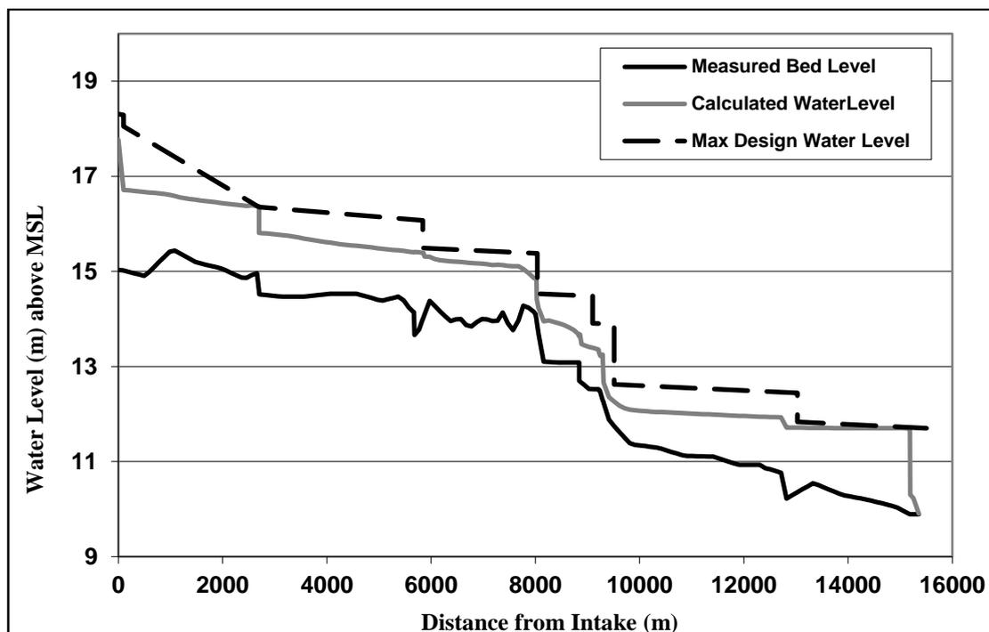
Figure 3: Computed water levels in scenario 1 versus design water levels of Bahr El-Gargaba
