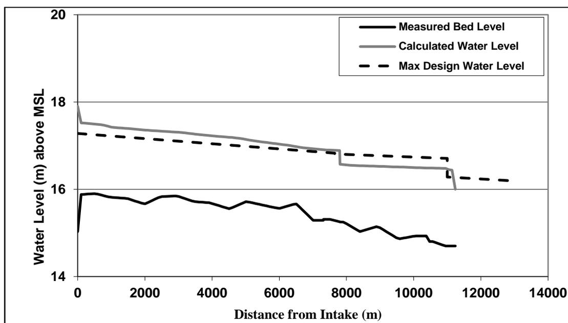
Figure 7: Computed water levels in scenario 2 versus design water levels of Bahr El-Bashawat
