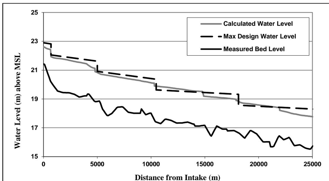
Figure 2: Computed water levels in scenario 1 versus design water levels of Bahr El-Gharq
