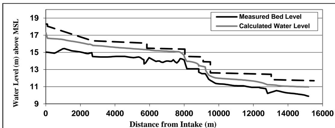
Figure 15: Computed water levels in scenario 5 versus design water levels of Bahr El-Gargaba
