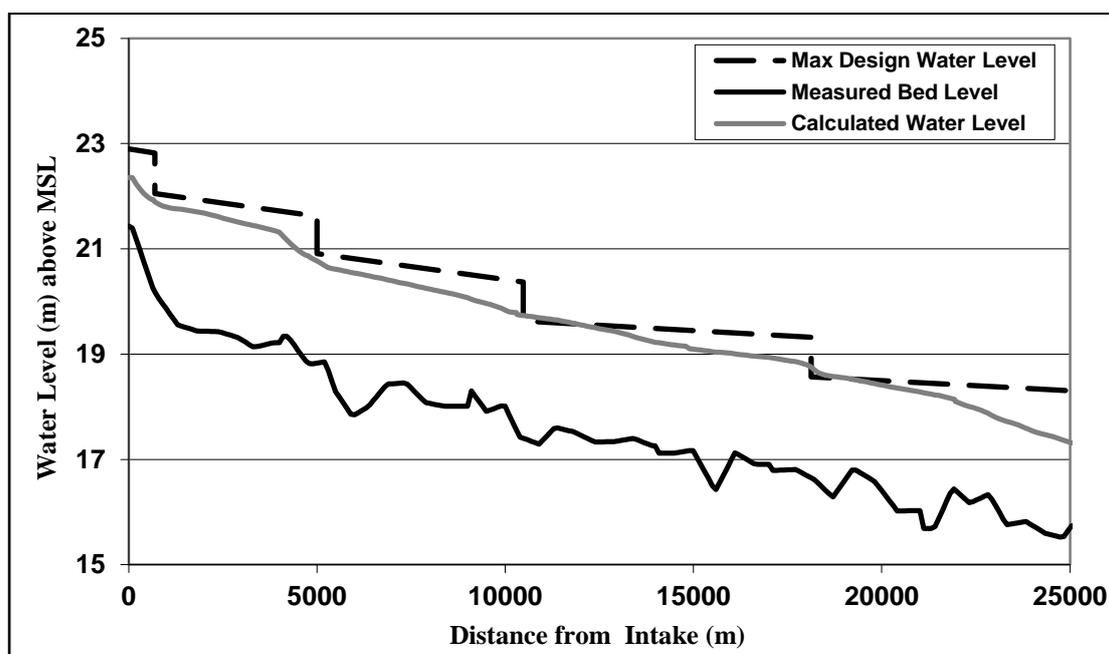
Figure 14: Computed water levels in scenario 5 versus design water levels of Bahr El-Gharq
